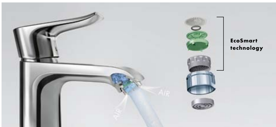
Thanks to EcoSmart technology, Hansgrohe wash basin mixers have a water consumption rate of just five litres a minute.
