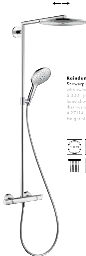
Raindance® Select E 300 Showerpipe for the shower with Raindance Select E 300 2jet overhead shower (17l/min), Raindance Select E 120 3jet hand shower (15l/min) and Ecostat Select thermostat, shower arm 380 mm # 27128, -000, -400
