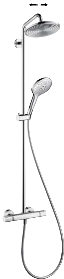
Raindance® Select 240 Showerpipe for the shower with swivelling overhead shower Raindance S 240 1jet (17 l/min), Raindance Select S 150 3jet hand shower (15 l/min) and Ecostat Comfort thermostat, shower arm 450 mm # 27115, -000 Height of the riser pipe can be reduced
