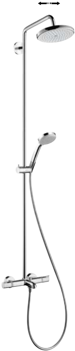
Croma® 220 Showerpipe for the bath with swivelling overhead shower Croma 220 1jet (16 l/min), Croma 100 Vario hand shower (15 l/min), Ecostat Comfort bath spout (20 l/min), shower arm 400 mm Height of the riser pipe can be reduced # 27223,-000
